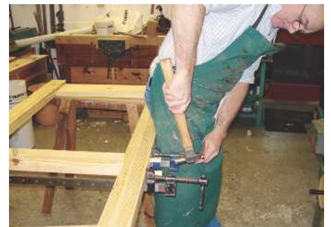
▲ Pic.9 The frame is now glued up, assembled, and the wedges are driven home
